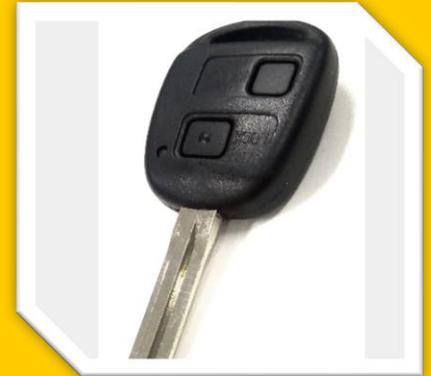
**NOTE:** You **MUST** have a working **BLACK** Master key to program your replacement Key to your vehicle otherwise a scan-tool will be required. The following procedure can be carried out without the new key being cut. Key blade requires cutting by a locksmith. Do not try to start the vehicle with the new key before it has been cut.
